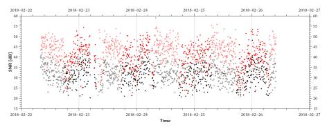
It is evident that the 128-chip code (red) gives a higher SNR than the 16-chip code (black). There also seems to be a slight difference between day-time (open symbols) and night-time (solid symbols).
