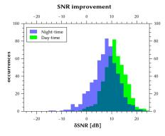
On average,  $\delta SNR$  (day) is 11.9 dB,  $\delta SNR$  (night) is 8.1 dB. Note: night-time distribution not completely symmetrical.
