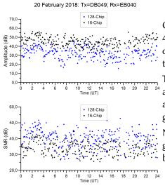
One day of highest SNR signals with 40 seconds integration time for the old sounding program, 20 seconds for the new one.
