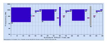
The current, day-time operations cycle for the Dourbes digisonde: total of 19 programs in 15 minutes, seven synchronised with EB040, four with JR055—getting very close to 100% of time usage.
